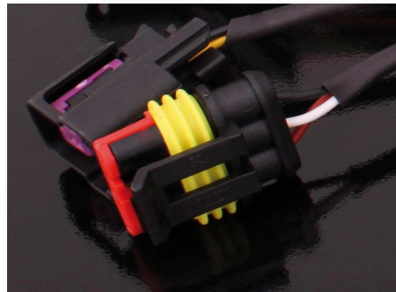
Fig 3 - 3-pin Superseal connector. 1: Signal GND. 2: AIN 4 (0-5V) input. 3: +5V from ECU.
